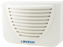
LS-652 / LS-652-1 Piezo siren Technical parameter 1.Operating voltage :12VDC 2.Rated current :130mA/120mA 3.Sound type: Single tone 4.Buzzer level :108±3DB/1M 5.Output power: 15W 6.Color :white 7.Package 100pcs/carton 8.CTN size :135x96x45mm .
