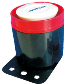
LS-653 Anti-theft alarm Technical parameter 1.Rated voltage:DC6V/12V/24V 2.Rated current:300mA 3.Output power:15w 4.Buzzer level:108±3DB 5.Sound type: one tone 6.color:black/white 7.product size:63.5*54*50mm
