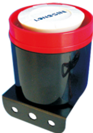
LS-653-1 Anti-theft alarm Technical parameter 1.Rated voltage:DC6V/12V/24V 2.Rated current:300mA 3.Output power:15w 4.Buzzer level:108±3DB 5.Sound type: one tone 6.color:black/white 7.product size:63.5*54*50mm
