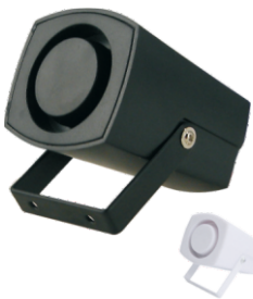
LS-651 Piezo siren Technical parameter 1.Rated current:300mA 2.Rated voltage:DC6V/12v/24v 3.buzzer level:108±3DB 4.Output power: 15W 5.color:black/white 6.product weight:0.05kg/pcs 7.Product size:58.6*42.5*38mm
